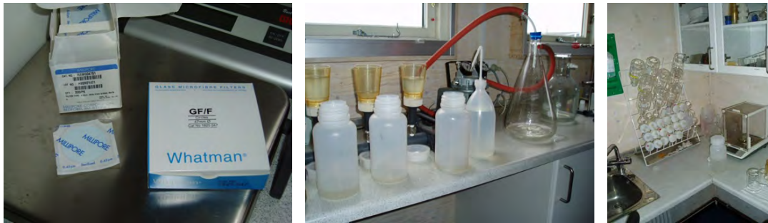
Figure 62: Whatman GF/F filters are used for filtration of suspended sediment samples (left). Milipore filter assembly connected to the vacuum pump. Three samples can be filtered at the same time (Mid). Analytical balance (right).
