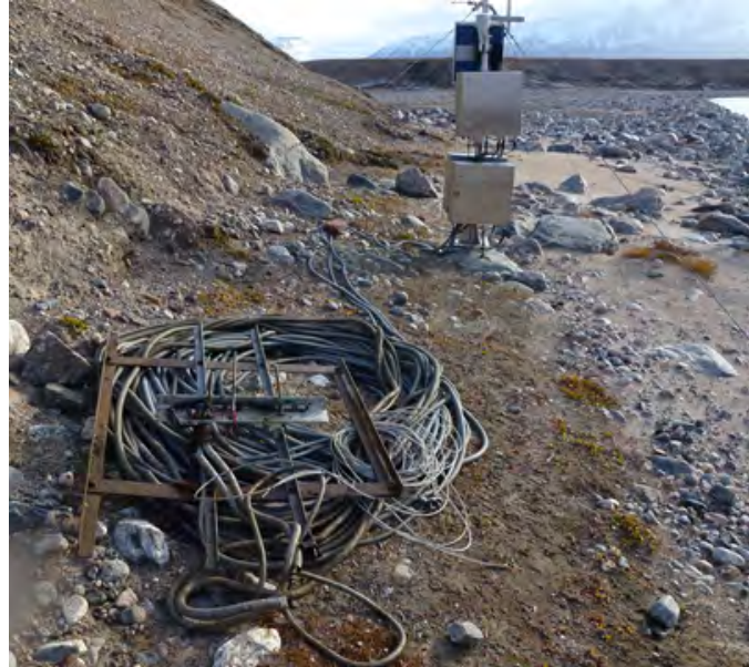
Figure 45: Storage of cable, frame and sensors during winter, by the old hydrometric station
