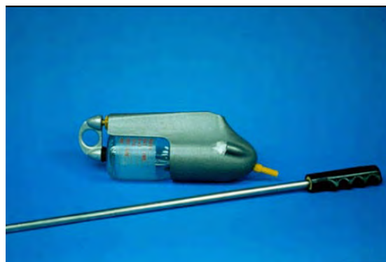
Figure 58: US DH-48 depth integrating sampler with 500 ml plastic bottles. To remove or insert the bottle; pull back and turn the handle in the back.
