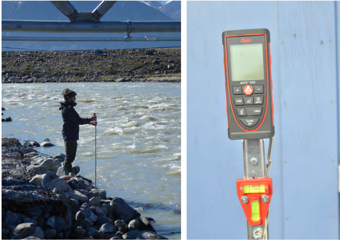
Figure 48: Measuring water table using the range finder and pointing it into the hoist trolley (left). Make sure the rangefinder is levelled using the small bobble level mounted on the pole (right)
