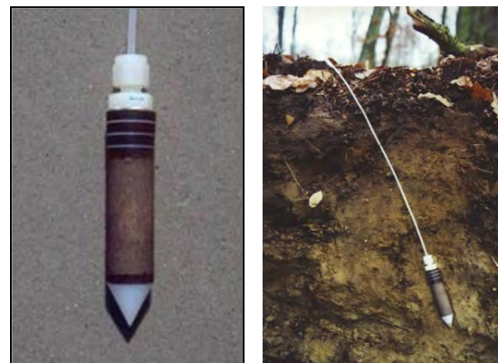
Figure 65: Left: Suction probe used in Zackenberg. Pore size: 2 microns. Right: Installed suction probe. A teflon tube connect the probe to the soil surface. Photo not from Zackenberg.
