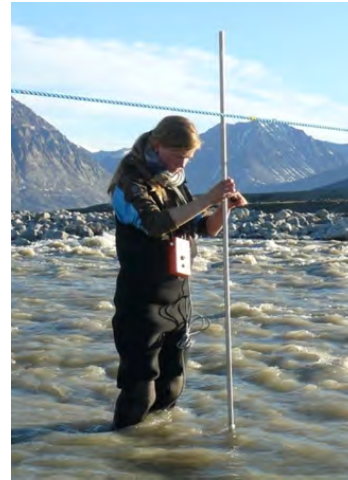
Figure 51: Standard velocity profile in the river and an example of measuring velocity at two different water depths.
