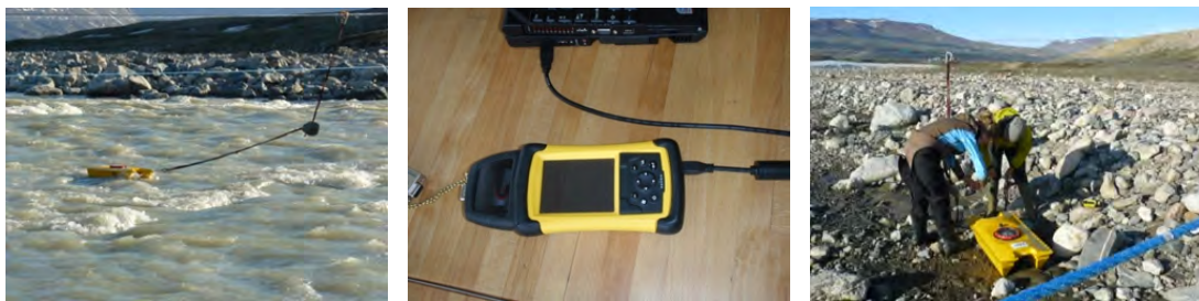
Figure 50: Q-liner boat in the river (left). PDA connected to computer (mid). Attaching the Qliner to the wire (right).
