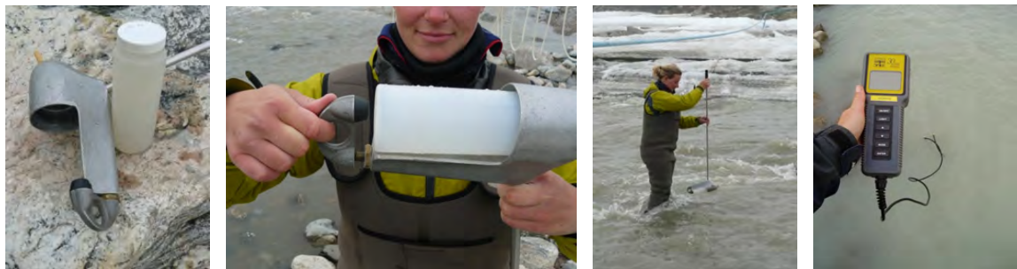
Figure 59: Depth integrating sampler and conductivity meter used during morning and evening sampling ([Update photo of conductivity meter in 2018!]).
