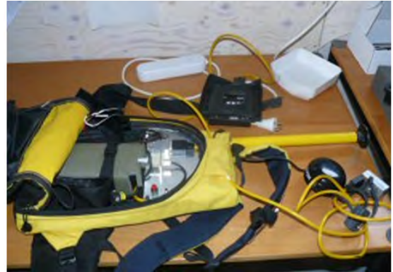
Figure 16: The data logger in the back pack with GPS antenna, cable and switch to mount on the probe.
