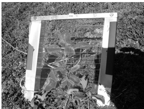
Figure 5.4. Maximum irradiance experiment, in which Salix arctica leaves are fixed in a position giving them maximum irradiance, covered by either UV-B-absorbing or UV-B-transmitting foil (Photo Teis N. Mikkelsen).
