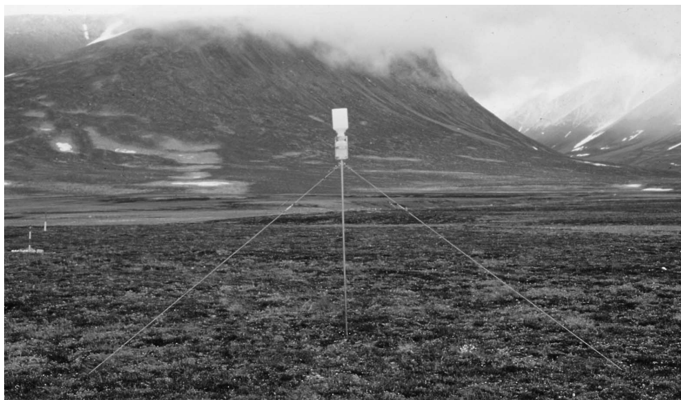
Figure 3.7. A mast for sampling of precipitation was erected near the climate station in 2002 (Photo Morten Rasch/ Polar Photos).
