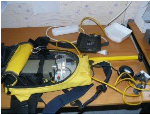
Fig 2.12 The data logger in the bag pack with GPS antenna, cable and switch to mount on the probe.
