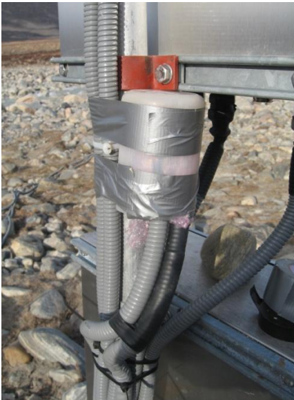
Fig 7.10 Detached cable/plugs stored during winter in the plastic bottle wired to the mast (left). All cable inlets to the data logger enclosure (right).
