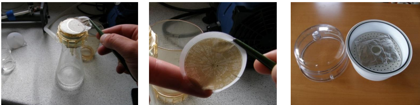
Fig 8.4 Moving filter with sediment from filter assembly to desiccator.
