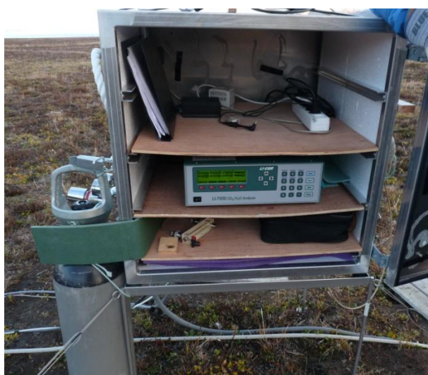
Fig 10.3 A look inside the enclosure, with the Licor7000, connected the eddy mast and the Nitrogen gas (on the left side of the enclosure) (left). A look inside the transformer box (right).
