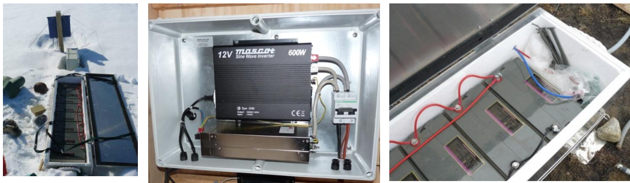
Fig 10.15 The battery box (left). A look into the transformer box, inside the hut (mid). Power cable from the instrument box enters the battery box in the southern end –the red and blue cable are connected to plus and minus on the last battery in the row.
