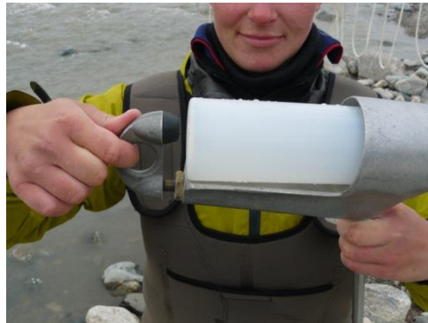
Fig 7.15 Depth integrating sampler and conductivity meter used at the daily sampling.
