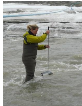
Fig 7.15 Depth integrating sampler and conductivity meter used at the daily sampling.
