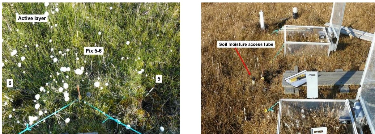
Fig 10.19 Looking down into the area in front of the chambers. Between the chambers there are fixed metal probes, use the top of these to measure the active layer (left). There are three soil moisture tubes between chamber 1-2, 3-4 and 5-6.
