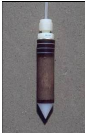
Fig 9.9 Suction probe used in Zackenberg. Pore size: 2 microns.
