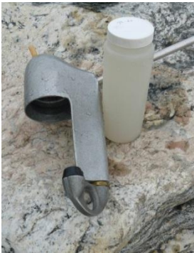
Fig 7.15 Depth integrating sampler and conductivity meter used at the daily sampling.
