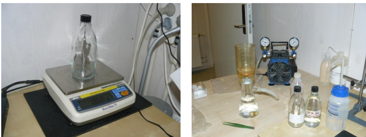
Fig 8.5 Pre-rinsed mercury bottle on the scale (left). Filter set-up (right).
