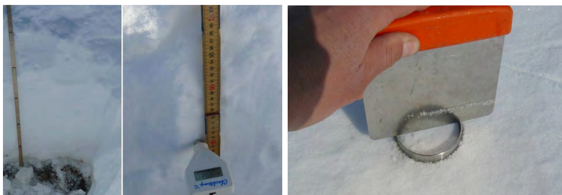
Figure 19: Snow pit without basal ice. Temperature recordings. Figure 20: A small ring (100 cm 3 ) is used to sample the surface snow.
