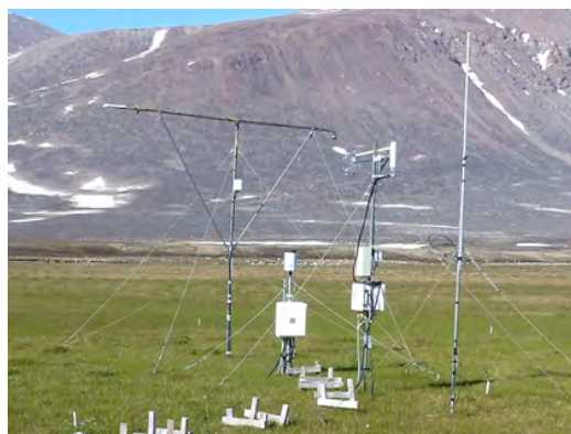
Figure 9: MM2 with energy balance mast, behind precipitation gauge and eddy covariance tower.
