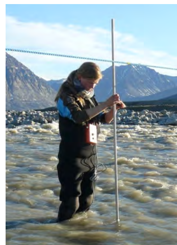
Figure 47: Standard velocity profile in the river and an example of measuring velocity at two different water depths.
