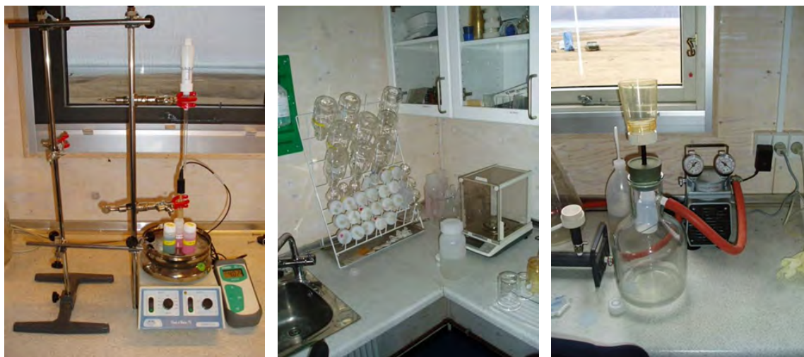
Figure 50: Laboratory in Zackenberg. pH meter next to the magnetic stirrer. The pH electrode is held by the lower clamp and the acid dispenser is held by the upper clamp (left). Analytical balance (middle). Device for filtration of water samples. Filtered water is collected directly into a clean sample bottle. Vacuum is applied by the electrical pump connected to the glass bottle (right).
