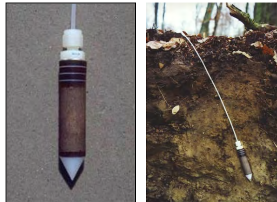
Figure 64: Left: Suction probe used in Zackenberg. Pore size: 2 microns. Right: Installed suction probe. A teflon tube connect the probe to the soil surface. Photo not from Zackenberg.
