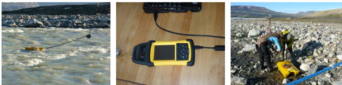
Figure 49: Q-liner boat in the river (left). PDA connected to computer (mid). Attaching the Qliner to the wire (right).
