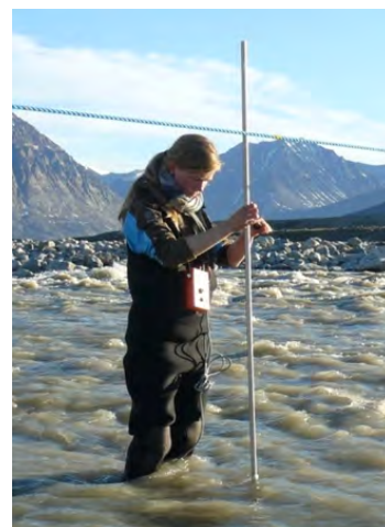
Figure 50: Standard velocity profile in the river and an example of measuring velocity at two different water depths.
