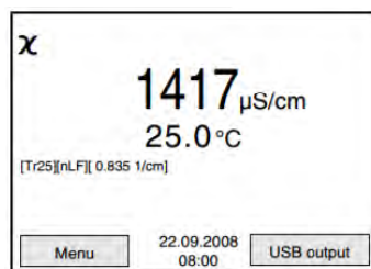
Figure 59: Display of cond3310 during measurement with nonlinear temperature compensation with a reference temperature of 25 degrees.
