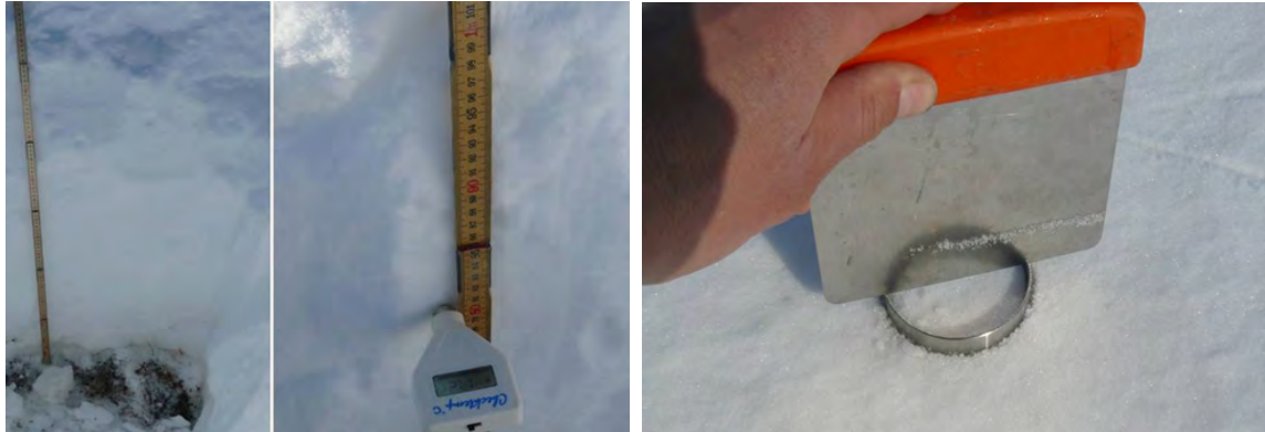
Figure 18: Snow pit without basal ice. Temperature recordings. Figure 19: A small ring (100 cm 3 ) is used to sample the surface snow.
