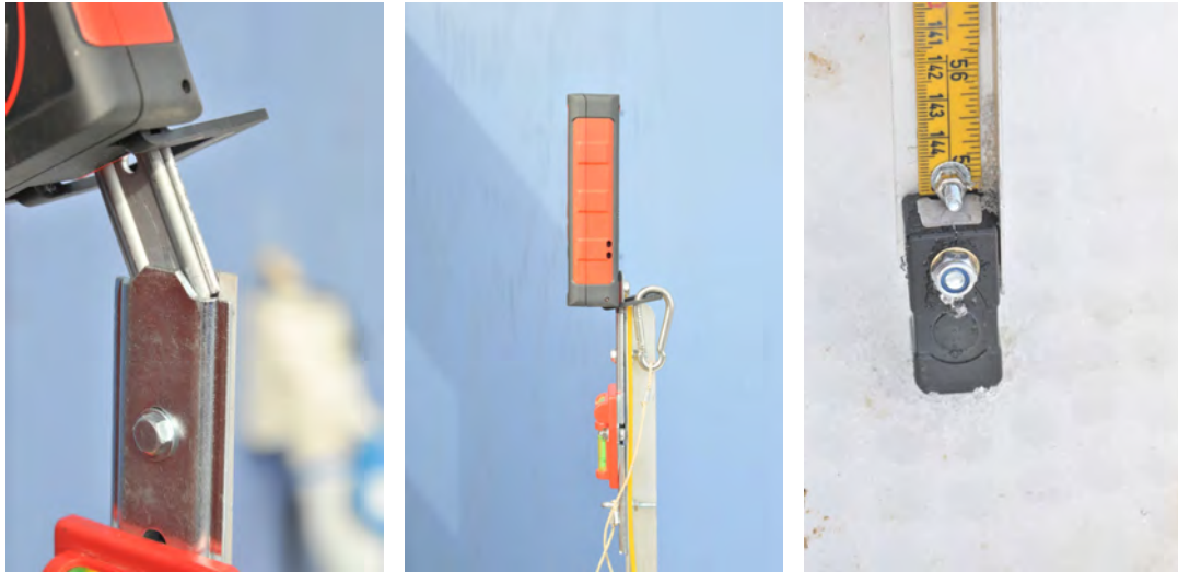
Figure 44: Correct mounting of range finder on pole with ruler (two leftmost photos) and placement of pole foot on a point directly under the hoist trolley (right photo).
