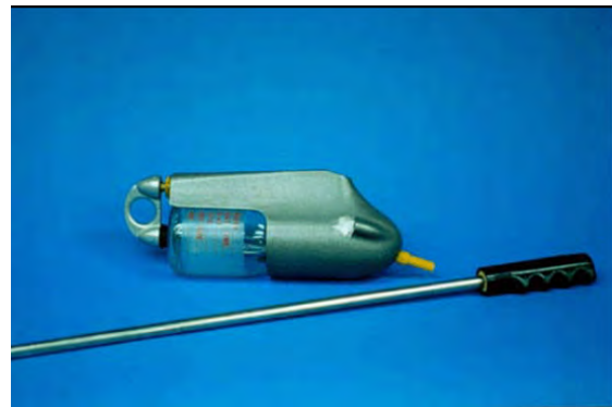
Figure 57: US DH-48 depth integrating sampler with 500 ml plastic bottles. To remove or insert the bottle; pull back and turn the handle in the back.
