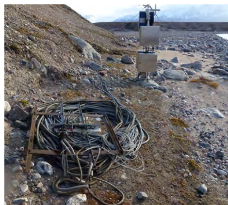
Figure 47: Storage of cable and sensors during winter, by the old hydrometric station
