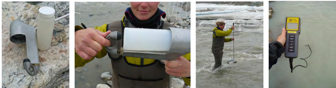
Figure 58: Depth integrating sampler and conductivity meter used during morning and evening sampling ([Update photo of conductivity meter in 2018!]).
